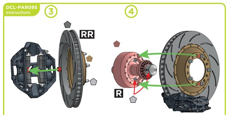
The left rear brake is assembled following the same steps as for assembling the right one, using the parts marked RL instead of RR.
