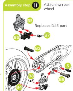
Place chain tensioner + caliper on swing arm replacing D45 part.
